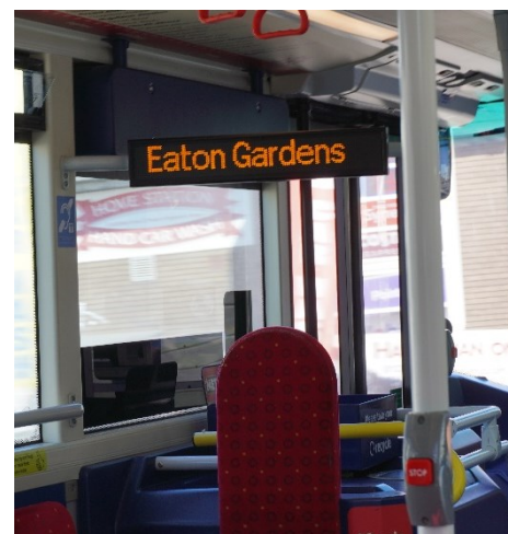
Figure 1 LED single line next stop display on a Brighton And Hove vehicle.
